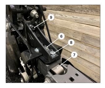
From the underside, maneuver the rock guard , with the guard extension to the rear, around the two side closing system bolts and align the rock guard bracket with the rear most hole in the 360 BANDIT extension bracket.
