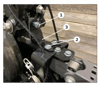
Remove the stop bolt ① and the remaining (2)  $3/8" \times 1-1/2"$  bolts and 3/8" flange nuts ② that secure the support strap ③ to the row unit and BANDIT arm assembly. Retain the (2)  $3/8" \times 1-1/2"$  bolts and 3/8" flange nuts.
