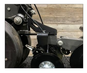
We have developed a different style of support bracket for BANDITS on White planters. This bracket provides more support for the closing system than the bracket provided with your BANDIT system last year.
