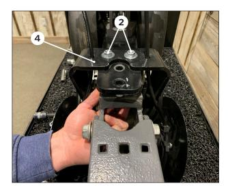
Keeping the BANDIT arm assembly in place 4 over the extension bracket and ensuring the BANDIT arms are facing the rearward direction, reattach the BANDIT arm assemble to the extension bracket using the (2) 3/8" x 1-1/2" bolts and 3/8" flange nuts 2 that were removed in the previous step.
