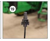
Install the push-to-connect fitting  $oldsymbol{\Phi}$  on the liquid tube on WAVE assembly.
