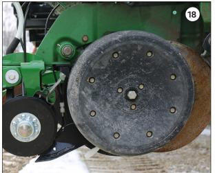
Reinstall right side disk and both gauge wheels using original hardware <sup>19</sup>.
