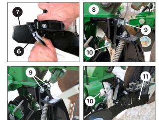
Install firmer (6) on the wave assembly (7) by pinching the top of the firmer together and slide it into place.
