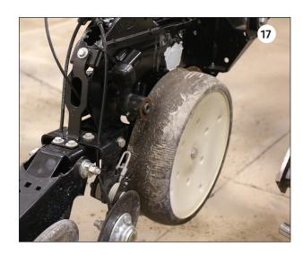
Reinstall right side disk and both gauge wheels using original hardware  $\mathbf{v}$ .
