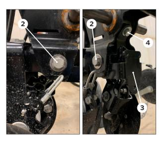
Back the nuts off of the bolts 2 that secure the BANDIT unit to the closing casting.
