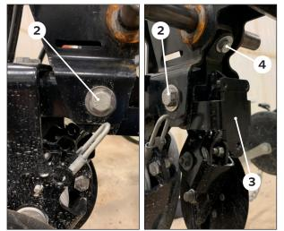
Back the nuts off of the bolts 2 that secure the BANDIT unit to the closing casting.
