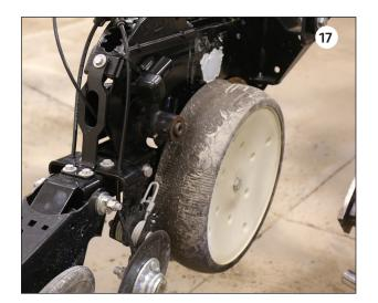
Reinstall right side disk and both gauge wheels using original hardware  $\mathbf{v}$ .
