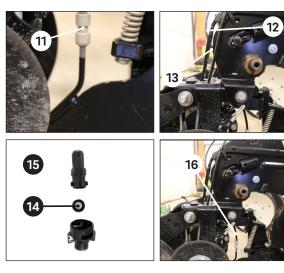
Install the push-to-connect fitting **1** on the liquid tube on WAVE assembly.
