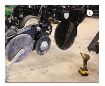
Remove both gauge wheels and the right-side opening disk **1**.
