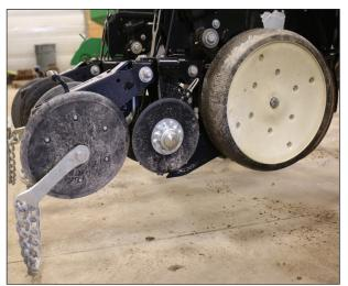
NOTE: Backing up when planter is not raised can cause wave blade to catch in the ground and bend or break. Use care to only back up after planter row unit is disengaged from the ground.
