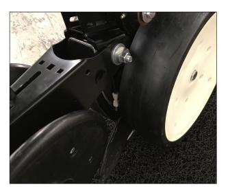
Reinstall right side disk and both gauge wheels using original hardware.
