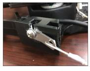
Insert screw through lanyard, and screw into tail of smart-firmer.
