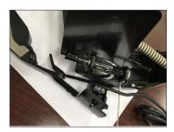
Route smart firmer cable as shown, then install smart firmer by sliding into firmer mount until it latches into place.
