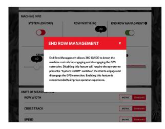
The system requires an inactive steering wheel and listens for **two presses** of the OEM auto-steer engagment button before it will engage 360 GUIDE steering. The 360 GUIDE system will automatically disengage when the steering wheel has been moved or if the sensors are not indicating incoming data.
