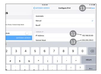
Once the "Manual" option is checked, a "Manual IP" section will appear in the window.
