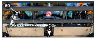
Route the longer section of harness 490233 with the 6-pin plug connector along the side and front of the cab to the sensor bracket .
