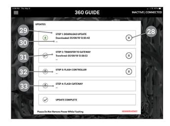
When the transfer is complete touch "STEP 3: FLASH CONTROLLER" ②. When complete step 3 will show a status of "Controller flashed".
