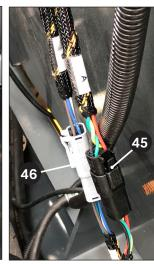
In the front dash panel, plug the 4-pin black male connector into the 4-pin gray female connector . This is the power source for the steering controller.
