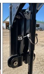
Mount steering breakaway 9 to the backside of the drop extension 6 using the 5/16" bolts, washers, and locknuts.
