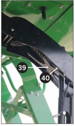
Feed the 6 pin plug end of the harness through the hole in the top of the sensor guard assembly and plug it in to the rear of the tactile sensor.
