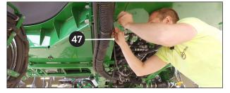
Connect the gray 12 pin connector on the harness to the gray port on the controller **5**. Use the extra black plug to fill the black port on the controller.
