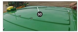
Plug in the 12 pin plug connector into the GPS port embedded into the front of the cab, just below the GPS globe and bracket . Secure the harness on the back of the GPS StarFire mount with a zip-tie, keeping it on the outside and bottom.
