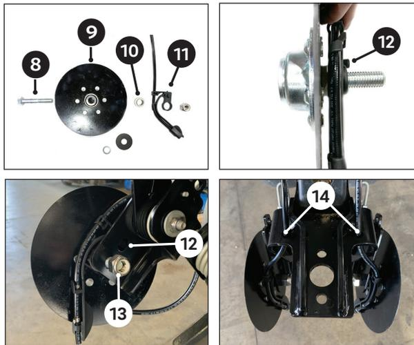
Insert 5/8" X 3" bolt **8** through the disk **9**. Place small shim washer then fender washer over the bolt. Insert bushing **10** (large side first) and hose guide assembly **11** (ear tab **12** facing in).
