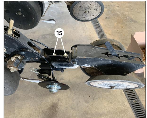
Using two remaining bolts and washers reinstall the closing system to the BANDIT unit **15**. Secure with nut.
