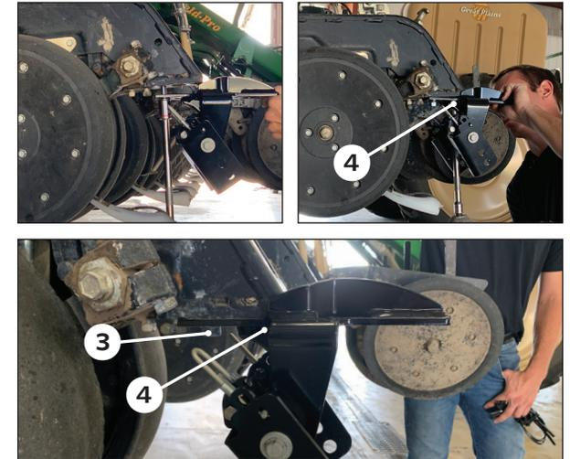
Using one of the long bolts ③ and one of the short bolts ④ from the provided hardware kit, attach the 360 BANDIT unit (long leg to the rear) to the row unit where the closing system casting was just removed. The longer bolt will be used in the front hole and the shorter bolt will be used in the rear hold.
