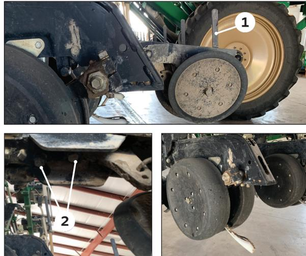
Release spring ① to remove tension from closing system.
