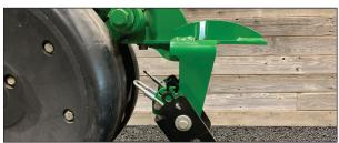
Using the two short M12 Bolts 4 attach the 360 BANDIT unit (long leg to the rear) to the row unit where the closing system casting was just removed.
