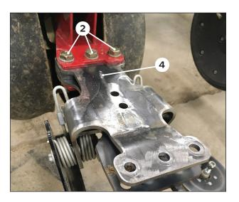
Slide the main BANDIT frame **4** in where the closing system was just removed. Loosely secure with the (3) 12 mm bolts, nuts, and washer previously removed **2**.
