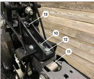
From the underside, maneuver the rock guard **10**, with the guard extension to the rear, around the two side closing system bolts and align the rock guard bracket with the rear most hole in the 360 BANDIT extension bracket.
