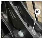
Align BANDIT arm assembly with the back horizontal holes on the extension arm.
