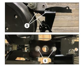
Using the two short 1/2" bolts ③ attach the 360 BANDIT unit (long leg to the rear) to the row unit where the closing system plate was just removed.
