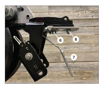
Insert one of the longer 1/2" bolts (3) through the rock guard (7) and then through the front hole on the closing system plate. Secure to the BANDIT unit.
