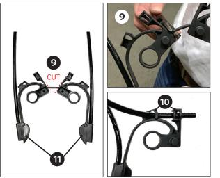
Using side-cutters, cut the two hose guides apart **9**.
