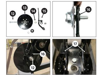
Insert 5/8" X 3" bolt 12 through the disk 13. Place small shim washer then fender washer over the bolt. Insert bushing 12 (large side first) and hose guide assembly 15 (ear tab 16 facing in).
