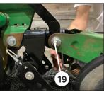
Attach the spring to the spring hook to on the extension bracket.
