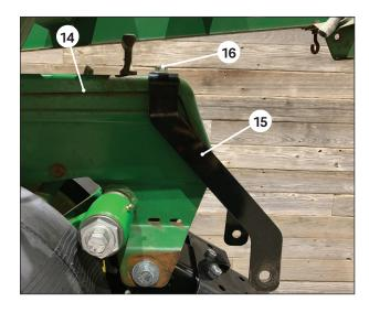
Using a 9/16" socket, remove the bolt from the top of the depth adjustment assembly and discard.
