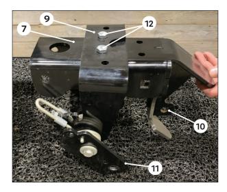
Slide the BANDIT arm assembly **9** over the extension bracket **7**. Ensure BANDIT arms **10** are facing in the rearward direction towards the spring hook **11**.
