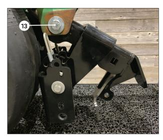
Align holes in extension bracket with the holes on the row unit. Install flat washer on  $\frac{1}{2}$ " x 1- $\frac{1}{2}$ " bolt from hardware kit #540615. Slide bolt through extension bracket and row unit hole (bolt head on the outside) **3.** Install another washer and hand tighten with nyloc nut from hardware kit #540615. Do not tighten.
