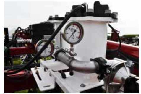
Centrifugal pump condenses NH 3 into liquid for even application, regardless of rate and temperature.
