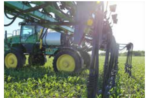
Breakaway mounting brackets and a flexible riser allow for easier navigation across hills and uneven terrain.
