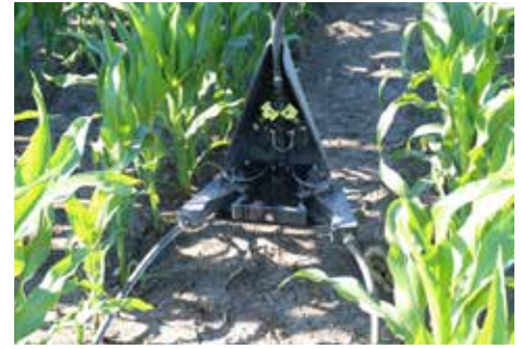
Four-position adjustable arms allow for precision placement in 15-inch to 36-inch rows and variable rate nozzles are available for precise rate control.
