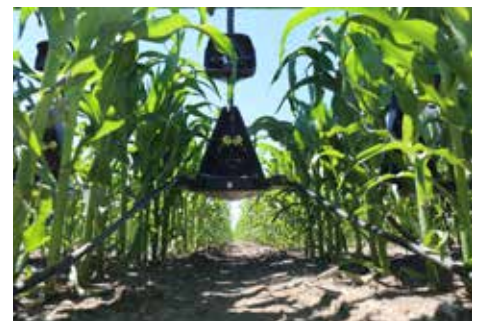
Curved hoses follow the corn rows and won't flop or "dance" which ensures nitrogen is delivered to the soil, not the stalk or leaves.
