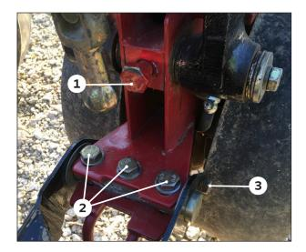
Remove (1) 16mm bolt (1), (3) 12 mm bolts (2) and stop bolt (3) to uninstall the closing system from the row unit.
