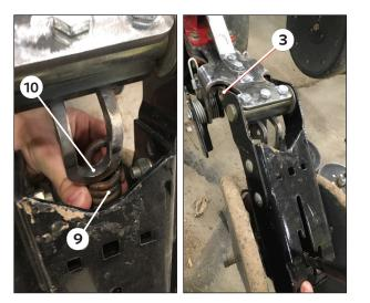
Attach the spring O from the OEM closing system to the hook O at the rear of the main BANDIT frame.
