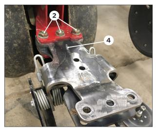
Slide the main BANDIT frame (2) in where the closing system was just removed. Loosely secure with the (3) 12 mm bolts, nuts, and washer previously removed (2).
