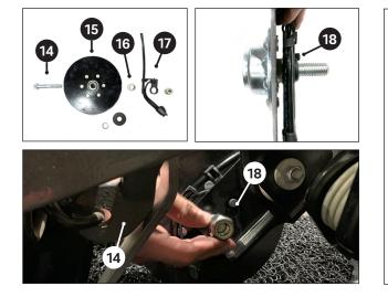
Insert 5/8" X 3" bolt <sup>12</sup> through the disk <sup>15</sup>. Place small shim washer then fender washer over the bolt. Insert bushing <sup>16</sup> (large side first) and hose guide assembly <sup>17</sup> (ear tab <sup>18</sup> facing in).
