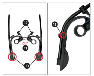
Using side-cutters, cut the two hose guides apart  ${f 0}$ .
