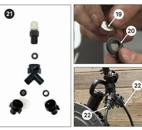
Install orifice plates 📵 in the rubber grommets 🕹.
