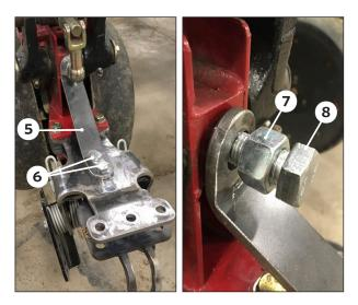
Place the support strap **5** on top the main BANDIT frame aligning the two holes in the strap with the two holes in the center of the main BANDIT frame.
