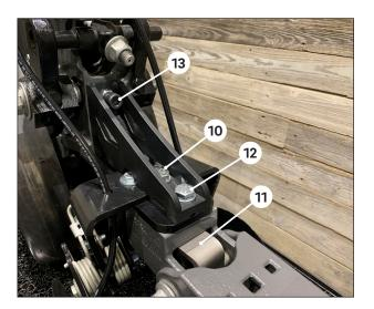
From the underside, maneuver the rock guard **①**, with the guard extension to the rear, around the two side closing system bolts and align the rock guard bracket with the rear most hole in the 360 BANDIT extension bracket.
