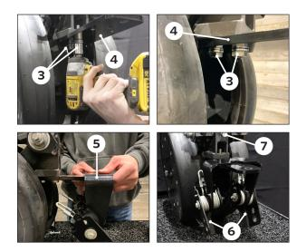
Using short M12 Bolts ③ install BANDIT extension bracket ④ (with BANDIT arm assembly installation holes to the back) using the closing system holes.
