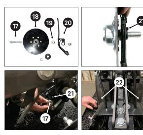
Insert 5/8" X 3" bolt 10 through the disk 18. Place small shim washer then fender washer over the bolt. Insert bushing 19 (large side first) and hose guide assembly 20 (ear tab 21 facing in).
