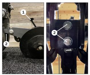
Release spring **1** to remove tension from closing system.
