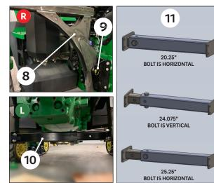
Using a forklift and strap, lift rear support ③ aligning hole in support with hole on the mount bracket.
