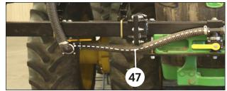
Install elbow on back of right side 2" fill valve with seal and hose clamp. Ensure hose barb is directed toward the center of the tractor.
