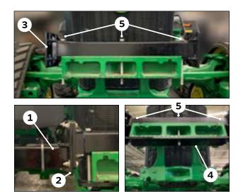
Set the front weight mount bracket ③ on top of the weight bracket with holes aligned with center hole of weight bar. Insert three bolts from the top to keep this bracket in place.
