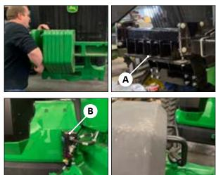
Remove weights. If your model has a short weight bracket it will need to be removed and replaced with a larger weight bracket and hardware provided by 360 Yield Center.
