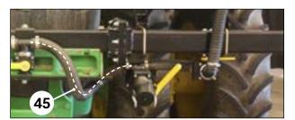
NOTE: Use lubricant as needed to slide hoses onto hose barbs.
