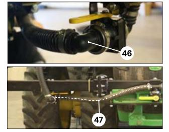
Install elbow 40 on back of right side 2" fill valve with seal and hose clamp. Ensure hose barb is directed toward the center of the tractor.
