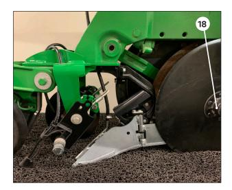
Reinstall right side disk and both gauge wheels using original hardware <sup>13</sup>.
