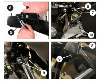
Install firmer **5** on the wave assembly **6** by pinching the top of the firmer together and slide it into place.
