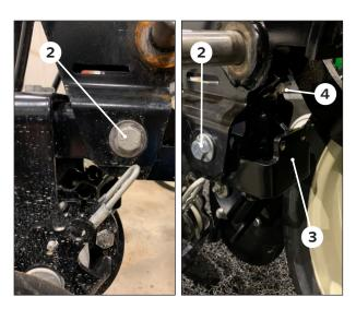
Back the nuts off of the bolts ② that secure the BANDIT unit to the closing casting.
