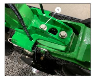
Using a 16mm socket and 19mm wrench, remove the front bolt ① that secures the 360 BANDIT to the closing system. The hardware should be retained as it will be reused.
