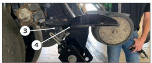
Using one of the long bolts 3 and one of the short bolts 4 from the provided hardware kit, attach the 360 BANDIT unit (long leg to the rear) to the row unit where the closing system casting was just removed. The longer bolt will be used in the front hole and the shorter bolt will be used in the rear hold.
