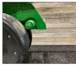
Release spring 1 to remove tension from closing system.
