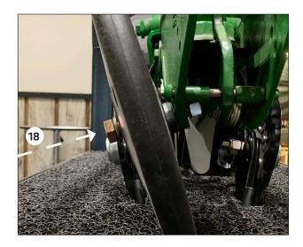
NOTES: If the closing wheels were removed but you are not installing the optional Chain Kit, reinstall the closing wheels at this time.
