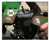
Insert 5/8" X 3" bolt 45 through the disk 46. Place small shim washer then fender washer 47 over the bolt. Insert bushing 48 (large side first) and hose guide assembly 49 (ear tab facing in).
