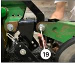
Attach the spring to the spring hook to on the extension bracket.
