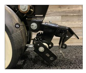
Align holes in extension bracket with the holes on the row unit . Install flat washer on the 1/2" x 1-1/2" bolt from hardware kit #540615. Slide bolt through extension bracket and row unit hole (bolt head on the outside). Install another washer and hand tighten with nyloc nut from hardware kit #540615. Do not tighten.
