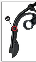
Remove the bolt on the bottom of the depth adjustment assembly and discard.
