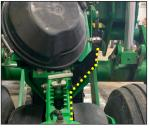
The two holes on the other end of the JD MaxEmerge 5 bracket 24 match up to the holes in the row unit casting.
