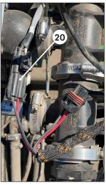
The DASH hub power harness has two branches of jacketed cable. The shorter branch (about 24 inches long) has a 2 position plug and a 2 position receptacle and this is how the hub gets battery power.
