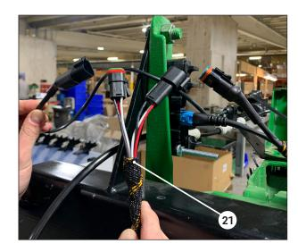
The longer branch (about 20 feet long) is how the hub gets switched key power. This branch should be routed to the nearest row. The end of this branch has a 3 position plug and a 3 position receptacle to split the flow meter connection on that row 2. The row harness and flow meter harness will be installed in a later step. There may be excessive cable length for the hub connections. A couple zip ties can be used to organize the excess cable.
