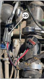
The DASH hub power harness has two branches of jacketed cable. The shorter branch (about 24 inches long) has a 2 position plug and a 2 position receptacle and this is how the hub gets battery power.
