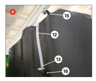
Apply white thread sealing tape to threads on each of the elbow hose fittings.
