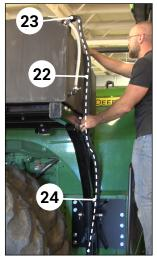
Install bottom 1-1/4" fitting into bulkhead towards the rear of the tank 20. Screw down to tighten and ensure port is faced to the rear.
