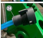
On the top of the BANDIT frame, locate the hole that was previously used to route the BANDIT hose. Install the new hose holder on top of that hole using the provided hardware. Ensure there is a washer on both top and bottom.
