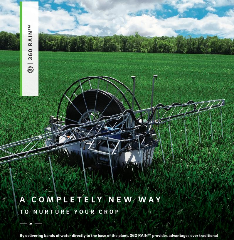
By delivering bands of water directly to the base of the plant, 360 RAIN<sup>TM</sup> provides advantages over traditional irrigation methods. 360 RAIN requires much lower volumes of water than traditional irrigation systems. Depending on field size, wells need to provide just 100 to 225 gallons per minute to the system. Plus, 360 RAIN can water irregular shaped fields that do not fit typical center pivot systems.
