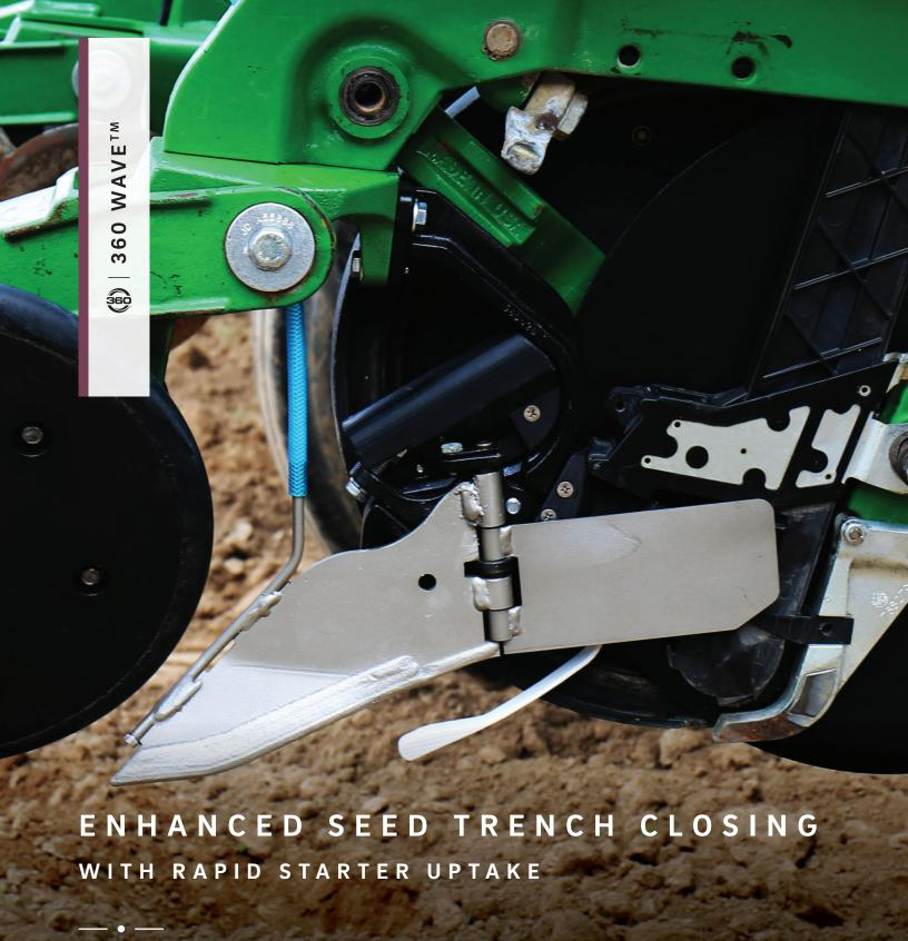
Surrounding corn seeds with moist soil ensures uniform emergence. And uniform emergence leads to better yields. 360 WAVE™ gently surrounds seeds by peeling a band of moist soil from the lower half of the seed trench and rolling it over the seed. That reduces risk of slotting and air pockets in dry, wet and ideal seedbed conditions.
