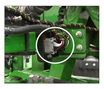
Plug the 12-pin plugs from the main harness into the controller.
