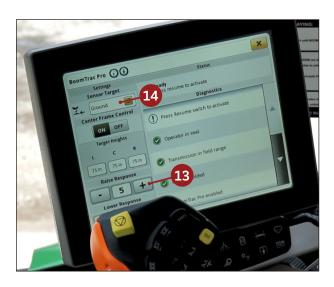
The raise response rate (13) can be adjusted according to your preference by clicking on the "-" or "+" buttons on either side of the numerical value in the "Raise Response" section. The higher the number, the faster the response.
