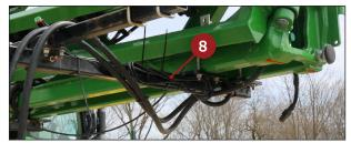
NOTE: The main harness has left, center and right specific connections. Ensure that each respective connection is routed to the correct side of the machine. Right and left are determined from the operators seat.
