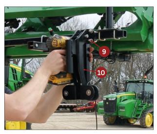
NOTE: If previously installed, 360 Y-DROP breakaways at the drop locations at center of the center section and the end of each primary boom MUST be removed and replaced with the new three-magnet breakaway.
