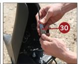
Using the drop harness (419312), plug the 4-pin receptacle connector into the previously routed boom harness Plug the 2-pin plug connector into the 2-pin receptacle connector on the three-magnet breakaway 3.
