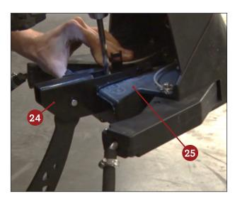
Slide the boom height base mount assembly 49 on your 360 Y-DROP base 45 from the back. Center directly between the two arms of the Y-DROP.
