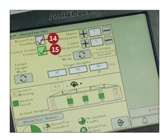
Ensure that both the "BoomTrac Enabled" 49 and the "Center Frame Control" 65 check-boxes are checked.
