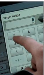
Click on the value under each sensor (L, C, & R) 12 to set the target height for each sensor location to match the reading from that sensor. E.g. if the actual sensor reading is a value of 75, the target height should be set to 75.
