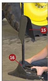
Install the risers • at each 360 GLIDE drop location by sliding the riser into the riser tube • on the three-magnet breakaway.
