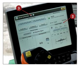
In the "Boom & Nozzles" window that opens, the boom height reading from the 360 GLIDE sensors is displayed to the right in the "Target Height" section 2.
