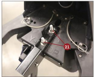
Insert 3/8" carriage bolts through the bottom of the base unit. Secure on top with washers and 3/8" nyloc nuts **2**. Tighten with 9/16" socket.
