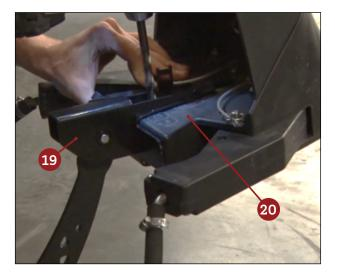
Slide the boom height base mount assembly <sup>19</sup> on your 360 Y-DROP base <sup>20</sup> from the back. Center directly between the two arms of the Y-DROP.
