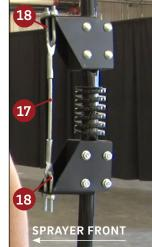
Install spacer blocks <sup>12</sup> by sandwiching riser above and below the spring. Ensure the nub on the block <sup>13</sup> goes into the indentation on the riser <sup>14</sup>.
