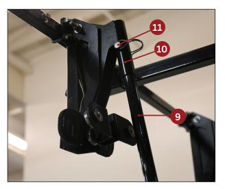
Install the risers **9** at each 360 GLIDE drop location by sliding the riser into the riser tube **10** on the three-magnet breakaway.
