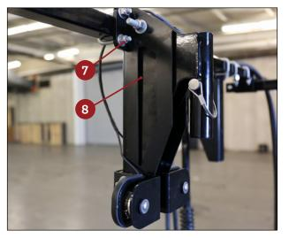
NOTE: If previously installed, 360 Y-DROP breakaways MUST be removed and replaced with the new threemagnet breakaway at the three 360 GLIDE drop locations.
