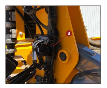
Plug the two 12-pin plugs from the main harness into the controller ③. Place controller in a safe location.
