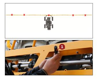
Unplug the five OEM Boom Height Sensors **1** located at the middle of the machine, each primary boom, and each secondary boom.
