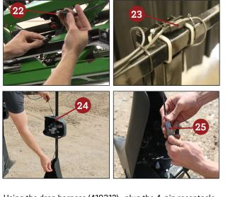
Using the drop harness (419312), plug the 4-pin receptacle connector into the previously routed boom harness <sup>(2)</sup> Plug the 2-pin plug connector into the 2-pin receptacle connector on the three-magnet breakaway <sup>(3)</sup>.
