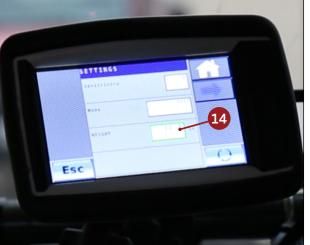
AGLEADER INTEGRA DISPLAYS ONLY: Set your measured height between 45-60 and match your target height to the measured height setting.
