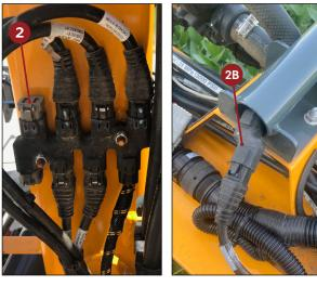
Plug the 12-inch harness adapter (419310) into the 4-pin receptacle connection of the main harness (419311).
