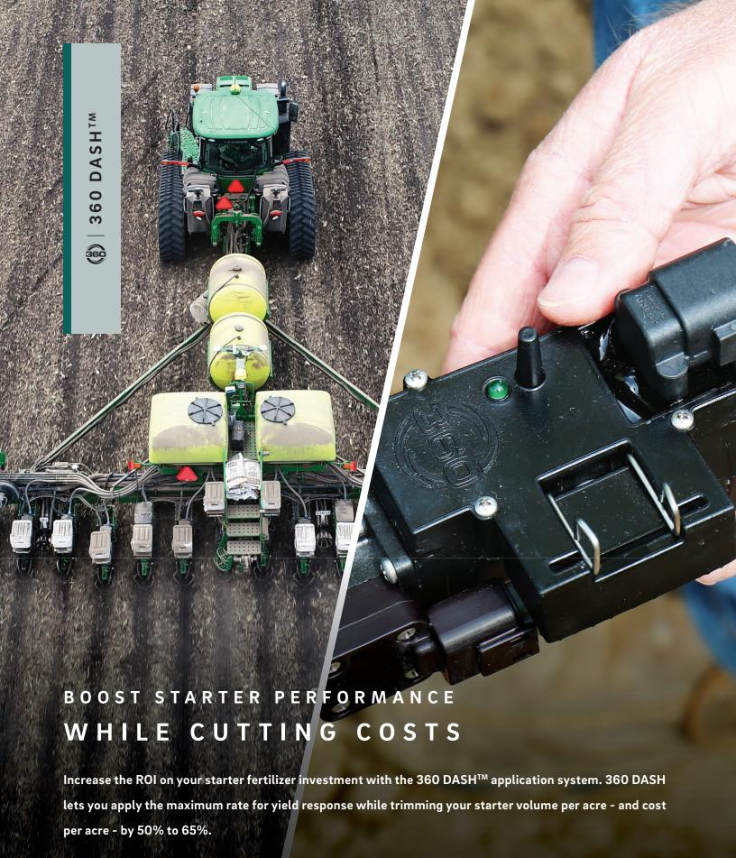
Rather than a continuous stream of liquid fertilizer, the 360 DASH valve meters a two- or three-inch "dash" of fertilizer and positions it for rapid interception by seedling roots.
