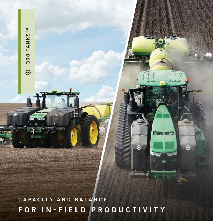
360 TANKS™ deliver the things you need for an efficient on-planter nitrogen system: weight balance, capacity, visibility and accessibility. These sleek 700-gallon capacity tanks follow the contour of the tractor - providing improved front and side visibility compared to other mid-mount and front-mount tanks.
