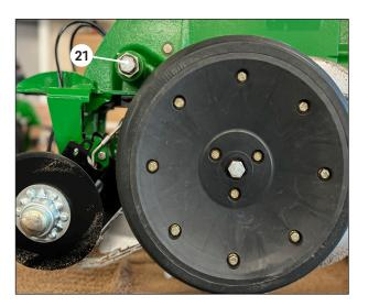
Reinstall both gauge wheels using original hardware **2**.
