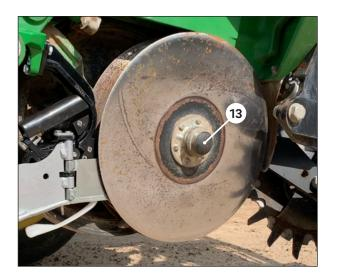
Reinstall right side disk using original hardware 13.
