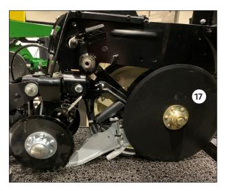
Reinstall right side disk and both gauge wheels using original hardware **1**.
