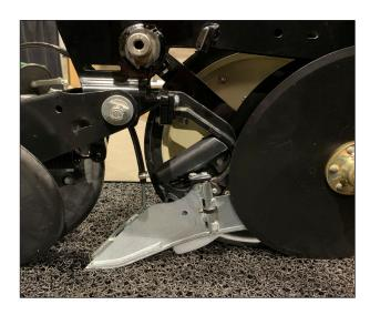
Reinstall right side disk and both gauge wheels using original hardware.
