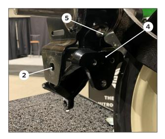
Install the provided closing casting 4 securing the top mounting location first using the provided 3/8" bolt 5.
