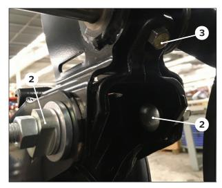
Remove the (2) carriage bolts ② and one regular bolt ③ that secure the closing casting to the row unit.
