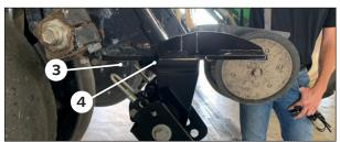
Using one of the long bolts 3 and one of the short bolts 4 from the provided hardware kit, attach the 360 BANDIT unit (long leg to the rear) to the row unit where the closing system casting was just removed. The longer bolt will be used in the front hole and the shorter bolt will be used in the rear hold.
