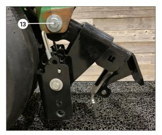
Align holes in extension bracket with the holes on the row unit. Install flat washer on  $\frac{1}{2}$ " x 1- $\frac{1}{2}$ " bolt from hardware kit #540615. Slide bolt through extension bracket and row unit hole (bolt head on the outside) **1**. Install another washer and hand tighten with nyloc nut from hardware kit #540615. Do not tighten.
