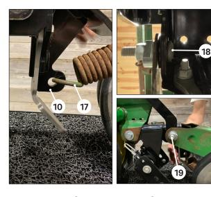
Attach the spring  ${f v}$  to the spring hook  ${f v}$  on the extension bracket.
