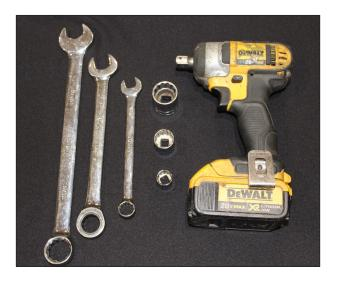
Hammer/Mallet Wrench Sizes: 3/4", 9/16" and 15/16" Socket Sizes: 3/4", 9/16" and 15/16" Impact
