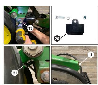
Tighten the nyloc nuts **1** that were left loose in STEP 3 with a ¾" socket and wrench, securing the BANDIT extension bracket to the row unit.
