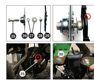
NOTE: Provided dust caps are matched with the hubs with which they are packaged. Keep each packaged kit together.
