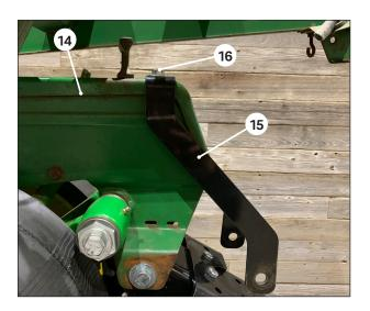
Using a 9/16" socket, remove the bolt from the top of the depth adjustment assembly <sup>10</sup> and discard.
