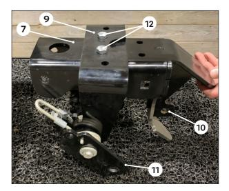
Slide the BANDIT arm assembly **9** over the extension bracket **9**. Ensure BANDIT arms **10** are facing in the rearward direction towards the spring hook **10**.
