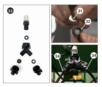
Install orifice plates 🗿 in the rubber grommets 🥹.
