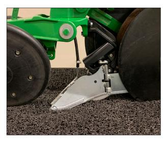
NOTE: When the planter is raised, contact between the WAVE blade and large spiked closing wheels is normal. During operation, the closing system comes up to operating depth and proper clearance is achieved.
