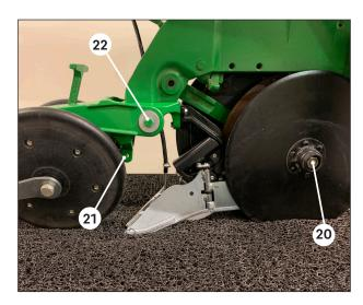
Route the 3/8" line through the hole  $\Phi$  on the row unit.
