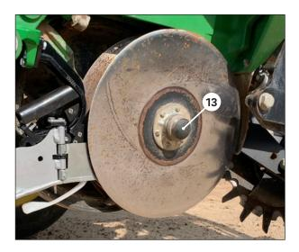
Reinstall right side disk using original hardware 13.
