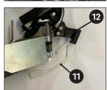
Apply lubricant to the bolts and threaded holes on the WAVE assembly and use a thread tap to clean out the holes.
