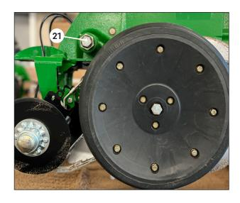
Reinstall both gauge wheels using original hardware 21.
