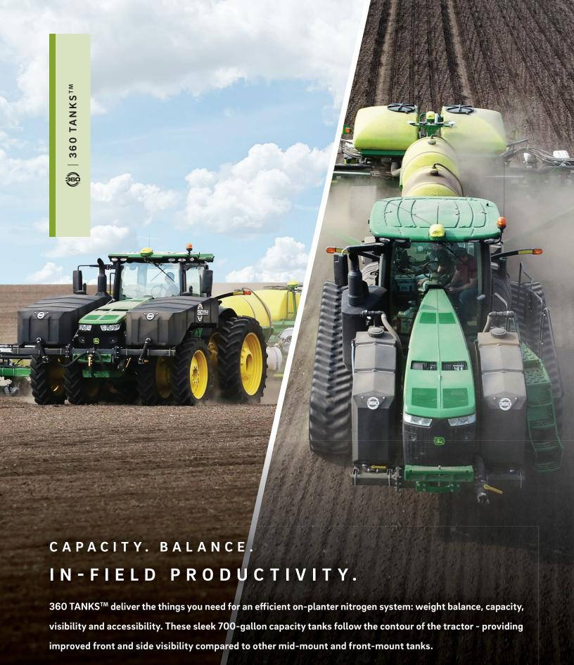
The unique shape and mount positions provide better fore-and-aft weight distribution to minimize pinch-row compaction. And, unlike most mid-mount tanks, 360 TANKS do not increase transport width.
