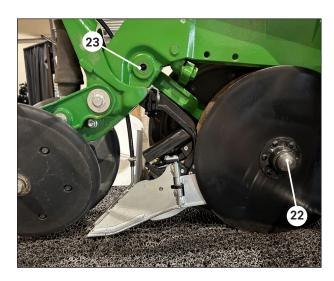
Reinstall right side disk 22 and both gauge wheels using original hardware 23.
