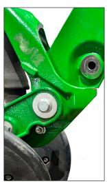
Using the hardware provided, reinstall the closing casting directly onto the shank by inserting one of the long bolts into the rear hole ② on the underside of the closing casing. Leave loose.
