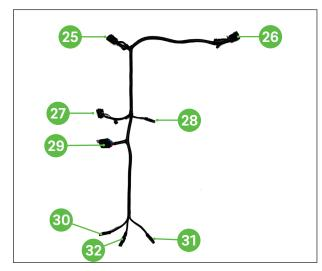
Locate the main harness with GPS connectors (part #575145).
