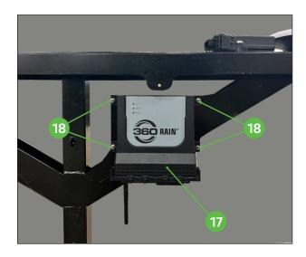
Install RCM Board (part #575500) 17 to the mounting location on the front left side of the planter tower using four M5 screws 18 provided in hardware kit #575758.
