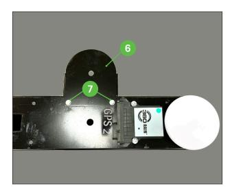
Install the antenna plate 6 to the front right side of the planter tower using the two shorter 1/4" bolts 2 from hardware kit #575758.
