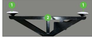
Install the two GPS receivers on top of the planter tower using the provided 5/8" bolts from hardware kit #575758. Tighten completely.
