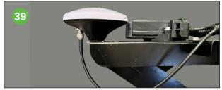
Connect one of the shorter coax cables with smaller connector (part #575185)  $^{35}$  to the GPS 1 receiver  $^{37}$ . Connect the other end of the cable to the GPS cable jax on the GPS 1 box  $^{33}$ .
