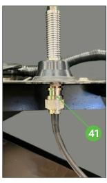
Connect the longer coax cable with the bigger connector (part #575142) 60 to the **GPS 1 box** at the 900 MHz post 40.
