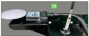
Connect the GPS 1 conector to the GPS 1 board directly behind the LTE device 25.
