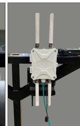
Carefully remove the four screws from the back of the LTE device. Keep these screws as they will immediately be used to install the device to the planter tower.
