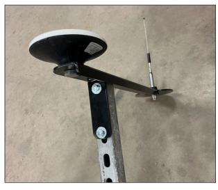
With the antenna mount assembled, it can now be secured to the base station structure.
